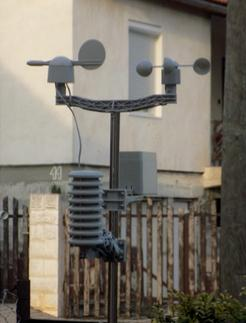
**Fig. 2.** Operating Bio Mosquito Trap (left) and the Velleman WS1080<sup>TM</sup> meteorological station (right).
